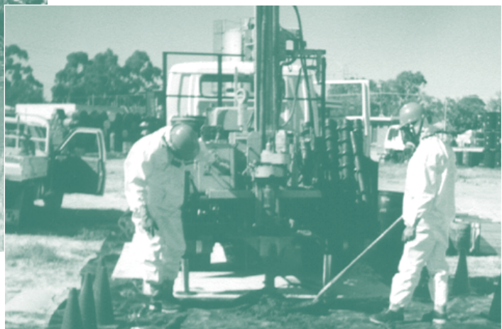
Groundwater in some areas has been polluted by industry or other land uses. The extent and severity of the pollution can be assessed by drilling and constructing monitoring bores.
